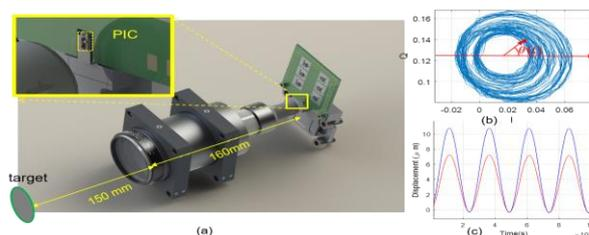
Figure 1: Figure. (a). Schematic show of the LDV setup with integrated PIC and confocal lens. (b) A Lissajous curve of the LDV output. The phase  $\theta(t)$  of each point is proportional to the measured displacement. (c) Recovered displacement signals at two different locations of a loudspeaker vibrating at 400 Hz.
