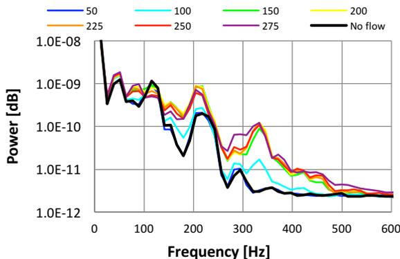
**Figure 3. FFT spectrum for a range of mean flow rates of accelerometer placed on phantom surface 20mm downstream from stenosis exit. Flow rates in ml/minute. LDV measurements on this system in progress.**
