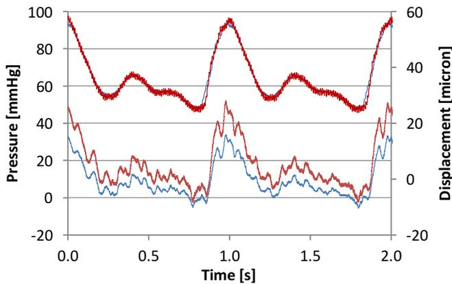
**Figure 2. Pressure within embedded tube (upper 2 traces) and displacement of phantom's surface (lower 2 traces) when subjected to pulsatile flow.**
